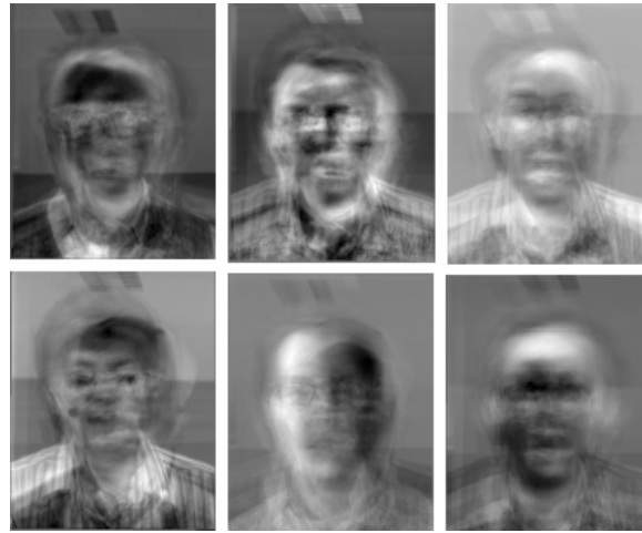
Fig. 11. Eigenfaces extracted from our training set that correspond to decreasing order of eigenvalues.
