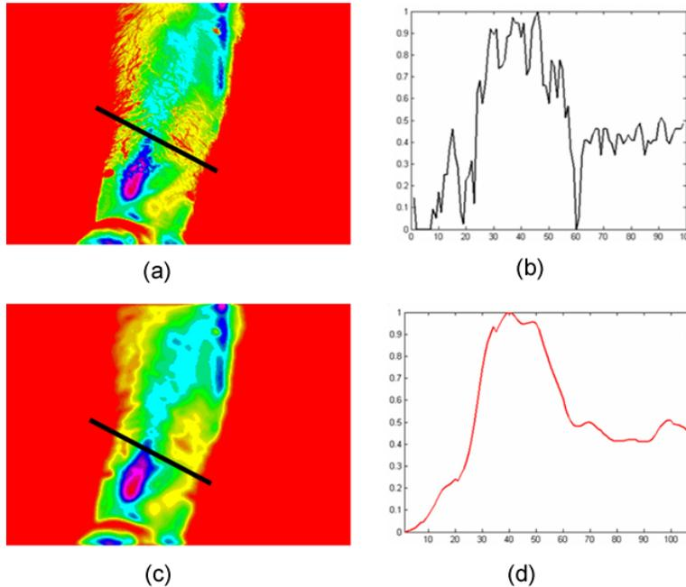
**Fig. 5.** Anisotropic diffusion on the thermal image of a human wrist: (a) Segmented wrist image; (b) profile of the line drawn across segmented image (shown in black color in (a)); (c) result of applying anisotropic diffusion on (a); (d) profile of the same line drawn across diffused image (shown in black color in (b)).
