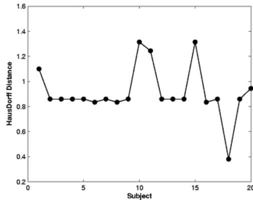
**Fig. 11.** Hausdorff distance plot between the automatically segmented and expertly delineated images.
