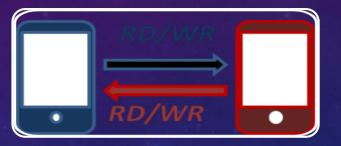
Active Communication Mode: Both Initiator and Target device communicate by alternately generating their own field. A device deactivates its RF field while it is waiting for data. In this mode, both devices typically need to have a power supply.
