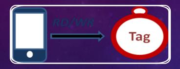
**Passive Communication Mode**: The Initiator device provides a carrier field and the target device answers by modulating existing field. In this mode, the Target device may draw its operating power from the Initiator-provided electromagnetic field.
