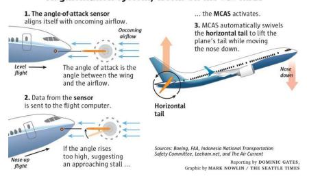
The tragic sequence of events on both flights began when a false reading from an AOA sensor activated a new flight-control system on the MAX — a piece of software called the Maneuvering Characteristics Augmentation System (MCAS) — that was designed, if the angle of attack got too high, to automatically push the jet's nose down uncommanded by the pilot.
