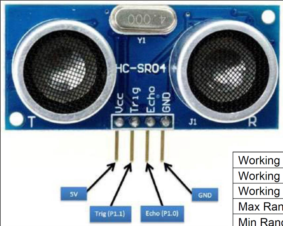
HC-SR04 ultrasonic sensor
