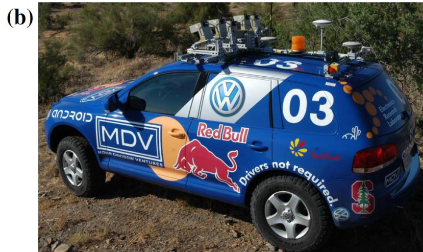
Figure 1: (a) The robot shown at approximately 1:40pm on Oct 8, 2005, as it successfully completes the 132-miles course. (b) View of the car and the roof rack with sensors. (c) The computing system in the vehicle's trunk.
