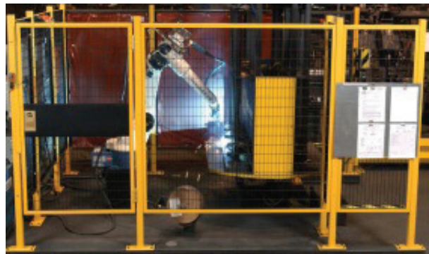
Figure 6. Robotic arm with a physical safety cage.
