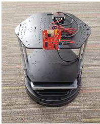
Figure 9. IWR1443BOOST EVM mounted on a Turtlebot 2.
