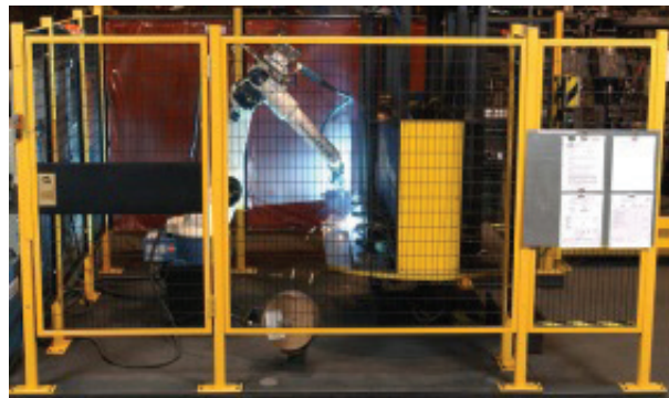
Figure 6. Robotic arm with a physical safety cage.
