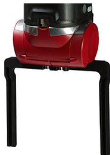
Figure 11 Baxter's Electric Gripper
