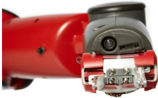
Figure 12 Baxter's camera and IR Sensor in the Cuff
