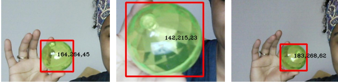
(a) Depth calculation from the calibration distance of 45 cm (b) Depth calculation when moving the ball closer to the camera (c) Depth calculation when moving the ball further from the camera
