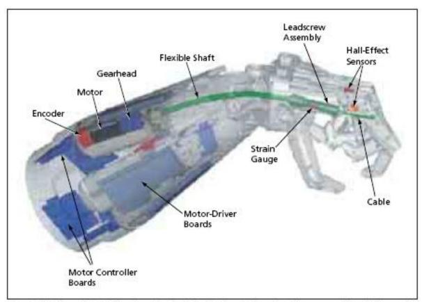
One of the Finger Drive Trains is emphasized in this view of the robot forearm and hand. The motive forces for the fingers are generated in the forearm and are transmitted to the fingers by flexible shafts, leadscrews, and cables.
