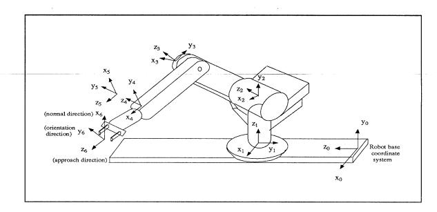
Fig 2. Scorbot - ER VII coordinates systems at various joints are shown.
