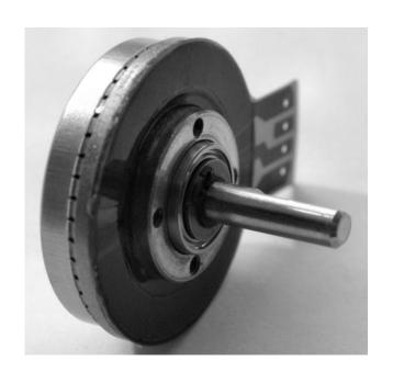
Piezoelectric Ultrasonic Motor
