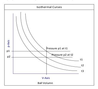
Each example isothermal curve corresponds to a different temperature (t1 > t2 > t3). For each constant temperature (t), pV = C, along the isothermal curve. The constant is larger the higher the temperature. The constant is not important in this example.
